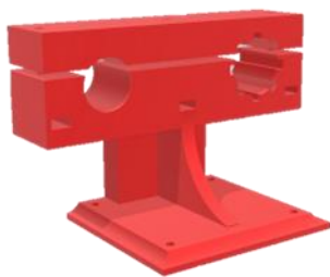
Fig-1: The Pumps' Mount
